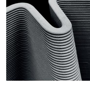
The project aims at developing new solutions for the design and manufacture of urban furniture by 3DP with ecological materials. Design and optimization of shapes will allow a reduction of mortar's quantity. Use of local recycled sand will slow natural resource depletion and avoid landfilling. Substituting natural constituents by recycled ones could reduce the regularity of the printed material and improving online monitoring during printing will allow to compensate the properties variability.
